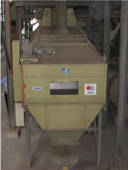
Photo 6 : Machinery to produce 100% OPF Cubes.
