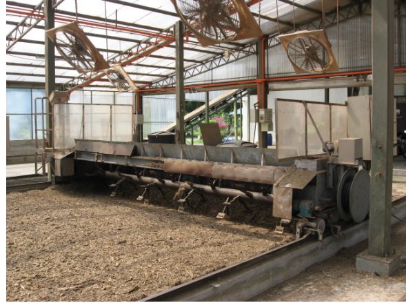
Photo 4: The OKADA system with improved flipping mechanism for drying shredded fronds using solar energy.
