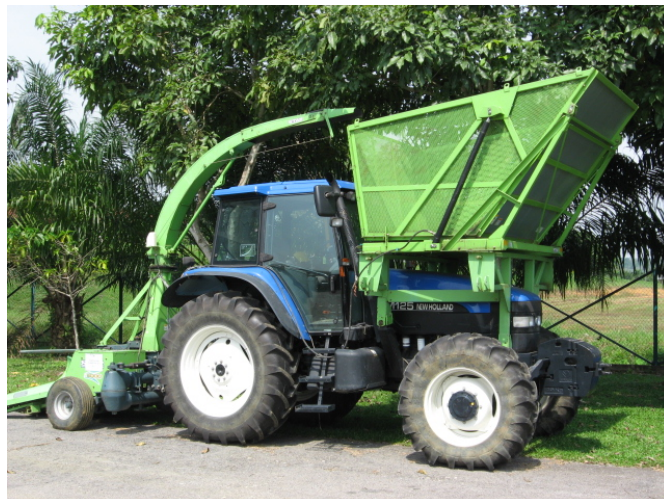
Photo 2: The oil palm frond 'auto-harvester' developed by the Project
