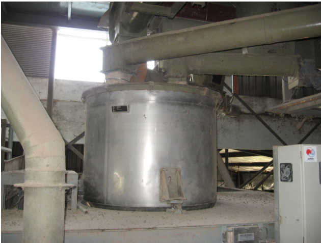
Photo 7: Mixer for mixing the dried OPF chips with other nutritional components such as rice bran, molasses, tapioca, PKC
