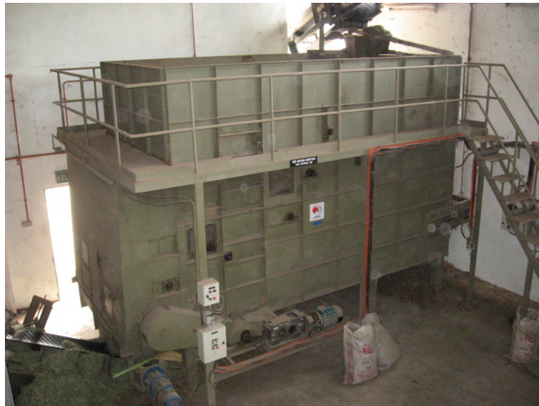
Photo 5: Dried chips are transferred by conveyor belt to this temporary storage bin before being stored in overhead silos.
