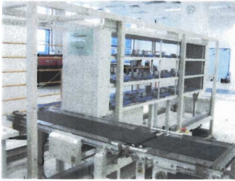
MFG5 - Automatic Warehouse (HAITECH SEIKO)
