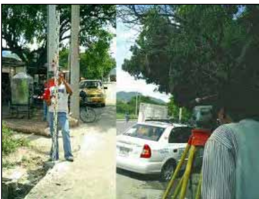
Figure 5-4 Ground Control Point Survey
