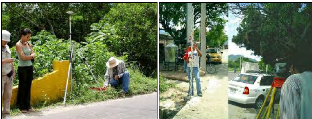
Checking of elevation data by direct leveling
