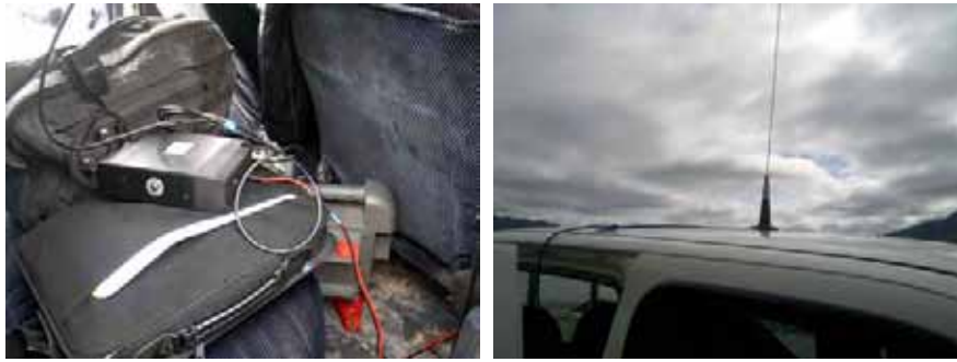
Fig. R 8.4.8 Mobile Radio (left) and Magnetic Mount Antenna (right)
