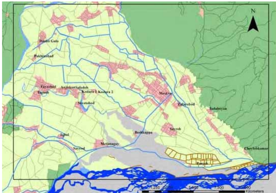
Fig. R 1.8.1 Boundary of Flood Inundation Simulations
