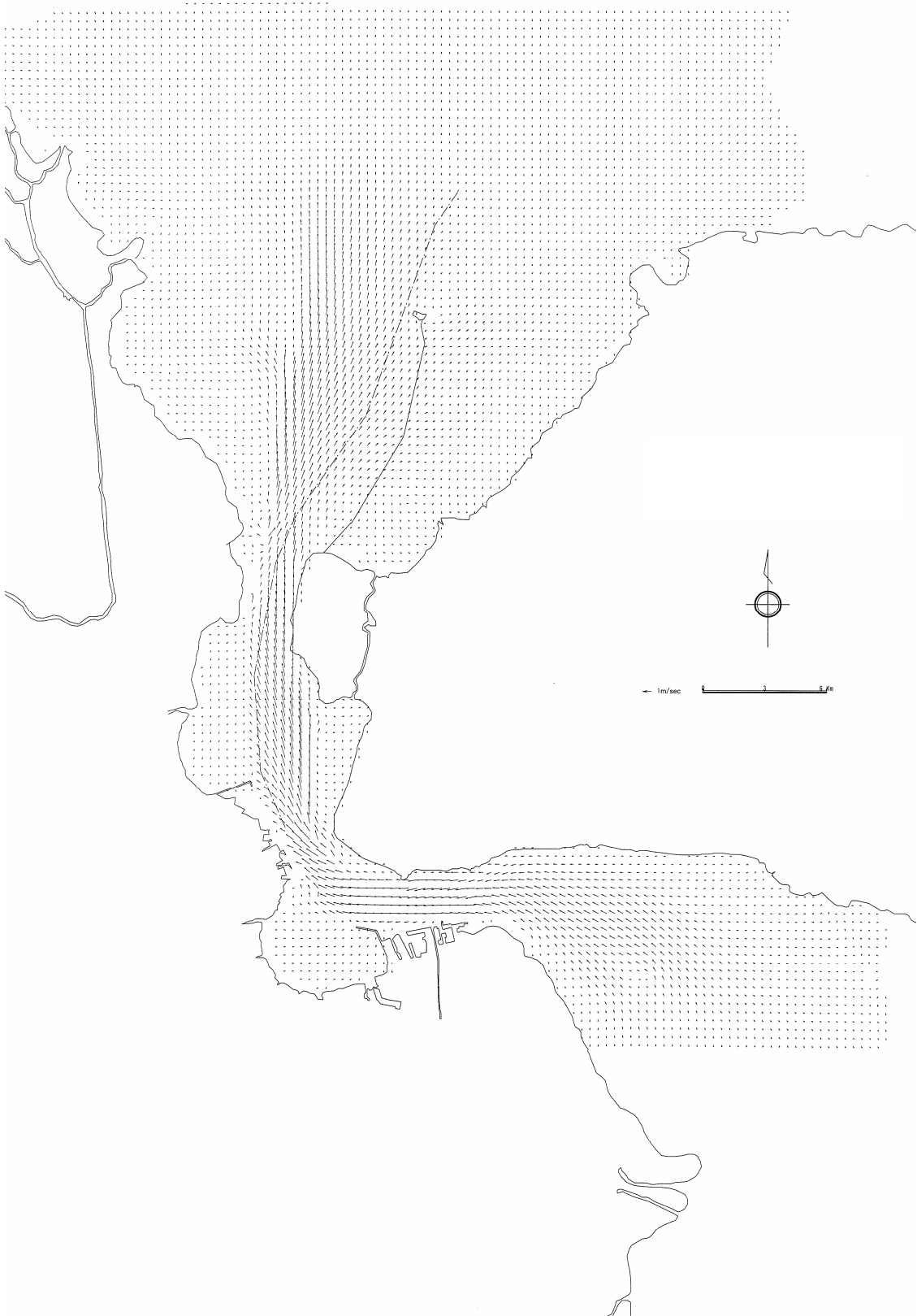
Figure A3.5 Currents of Upper Layer for the Maximum Flood Current in Rainy Season
