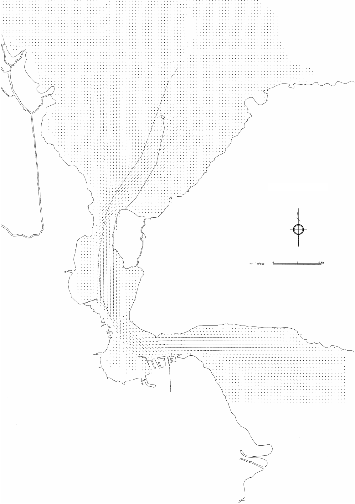
Figure A3.7 Currents of Upper Layer for the Maximum Ebb Current in Rainy Season
