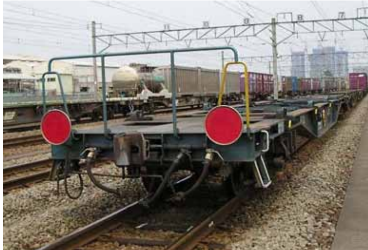
Figure 9-4 Container Wagons with Reflective Red Circle Substituted for the Brake Van (Japan)
