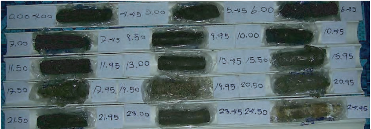
BH-J1, 26.0 m depth, Sea Water Depth 2.1 m, Feb 14-18, 07
