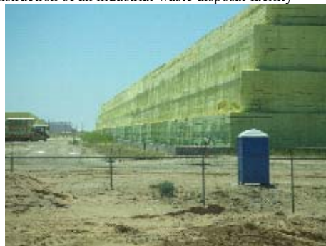
Storage condition of surplus sulfur
