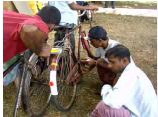
FIGURE 12- 1: RETRO-REFLECTORS FOR BICYCLES
