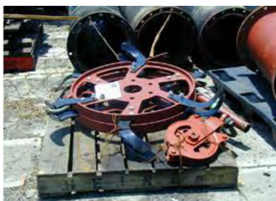
Components of side rotary type excavator on September 23, 2005
