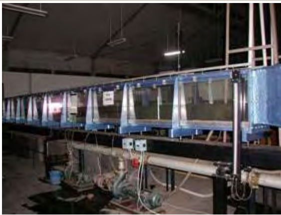
Experimental setup of flume sediment erosion test in Gaja Mada University, on November 11, 2004
