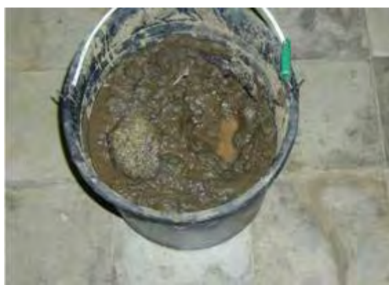
Remaining sediments in the receiver tank after Test on October 24, 2005
