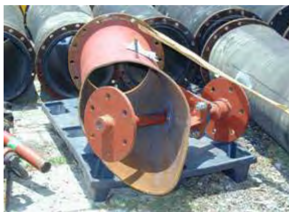
Components of water jet nozzle on September 23, 2005
