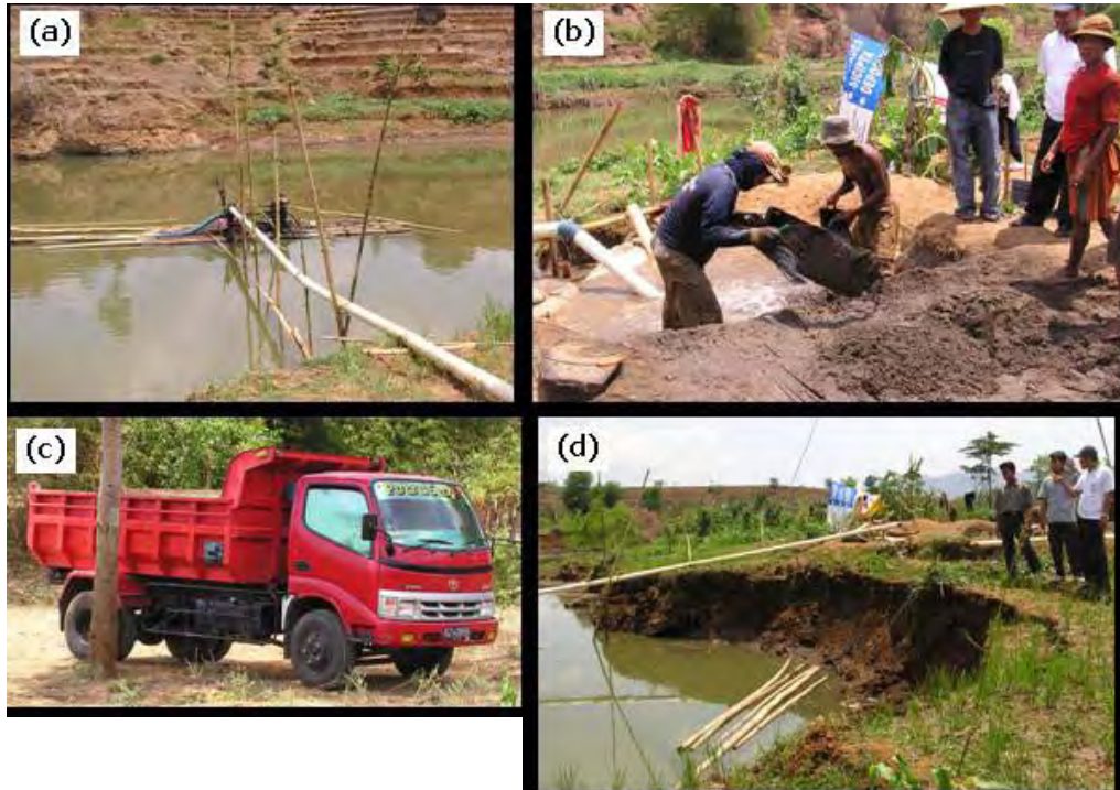
Location: Desa Pulosan, Kec. Wonokerto, Wonogiri, (a) Collecting Sand by motor pump, (b) Collected sand material, (c) Truck with a capacity of 4 m 3 and (d) Erosion on left and right sides of the river.
