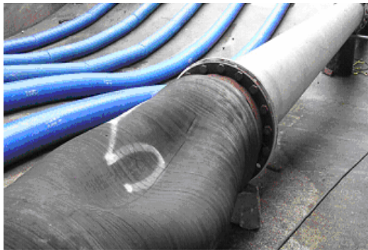
Photo 4.1.1 Deformation of the Rubber Flexible Joint
