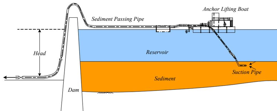
Figure 6.1.1 Schematic Profile of Hydro-Suction System
