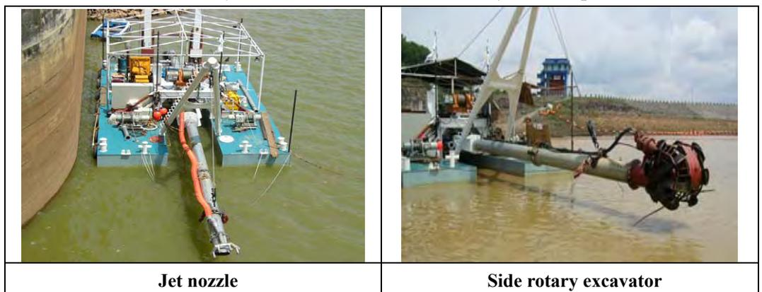
In case of jet nozzle, the performance was poorest among the three (3) types, because it was not possible to set the optimal angle between the nozzles and sediment surface due to the shallower dredging depth and operation in the water. The angle of the nozzles relative to angle of the suction pipe was a main issue to be solved in the future.
