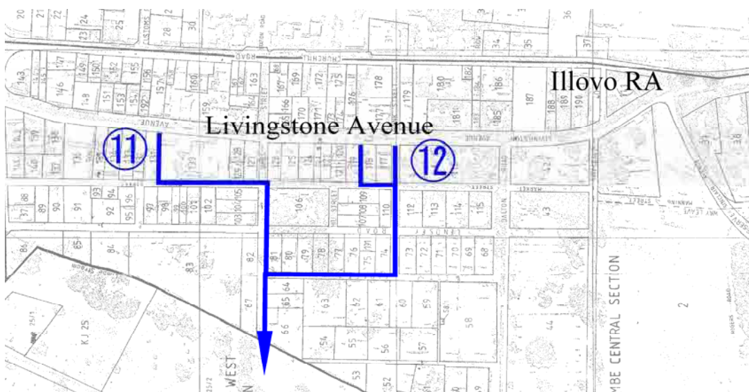
Figure 2.10 Drainage System on Livingstone Avenue (U Shape Gutter with Cover)
