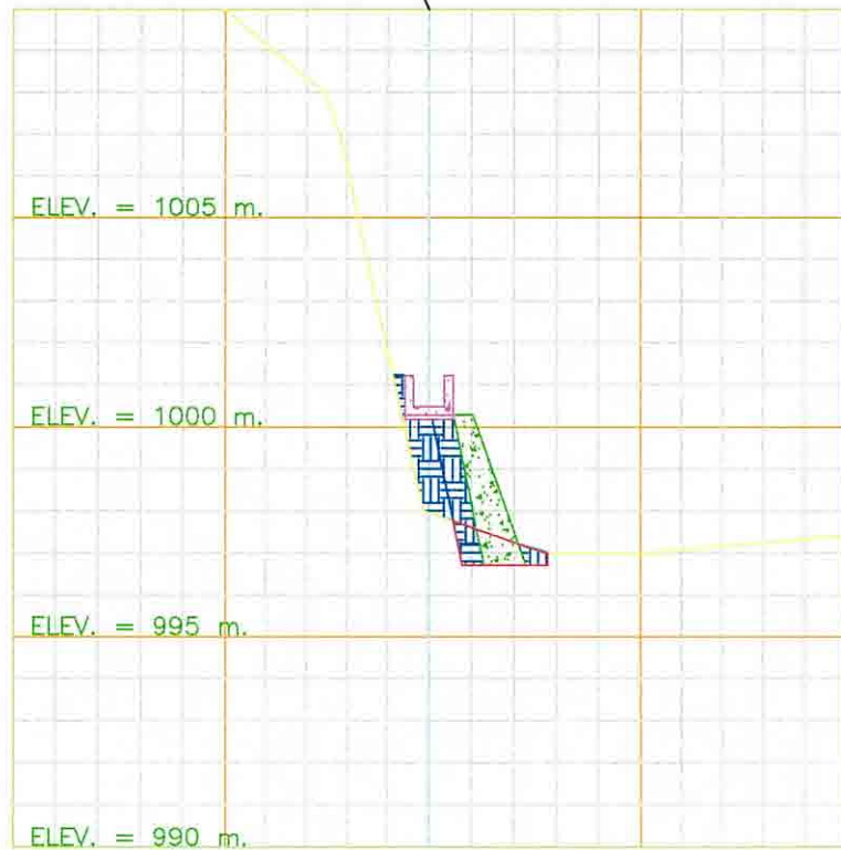
HEADRACE CHANNEL TYPICAL SECTION 1 (S = 1 : 100)
