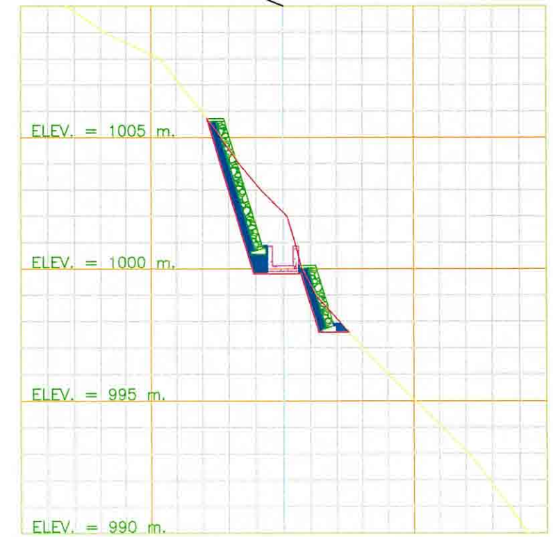
HEADRACE CHANNEL TYPICAL SECTION 6 (S = 1 : 100)
