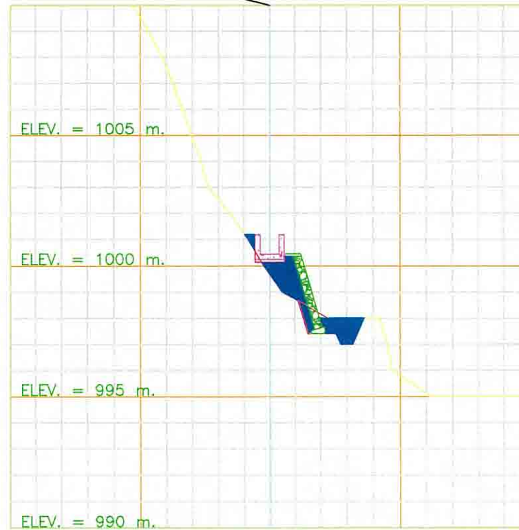
HEADRACE CHANNEL TYPICAL SECTION 2 (S = 1 : 100)
