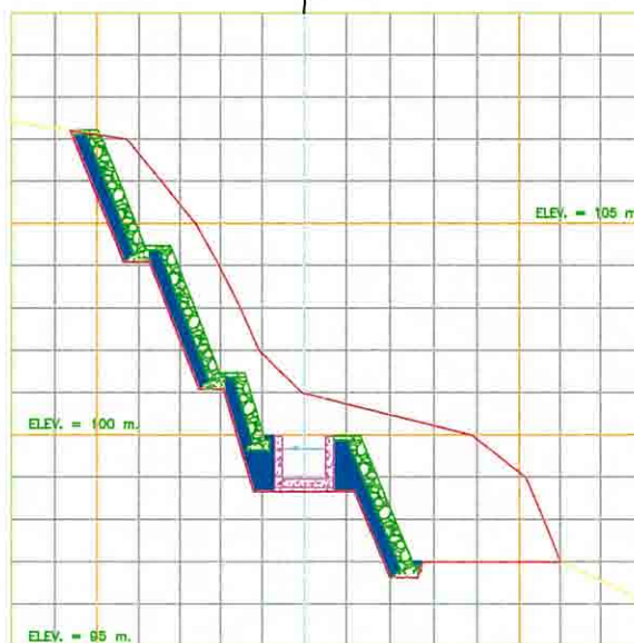
HEADRACE CHANNEL TYPICAL SECTION 1 (S = 1 : 100)
