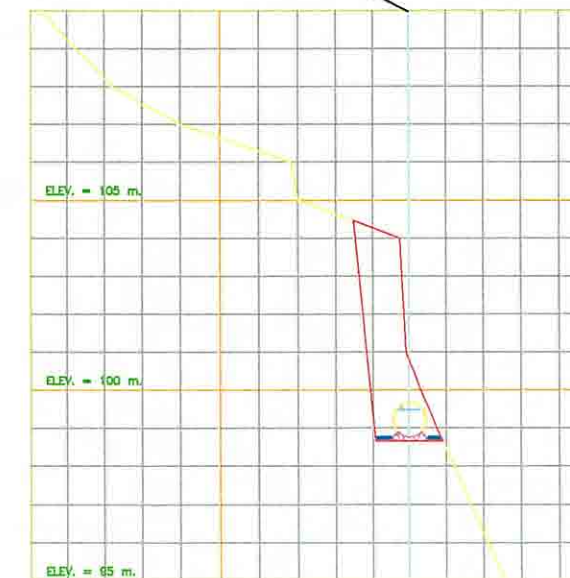
HEADRACE CHANNEL TYPICAL SECTION 3 (S = 1 : 100)
