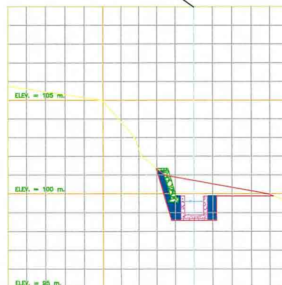
HEADRACE CHANNEL TYPICAL SECTION 2 (S = 1 : 100)
