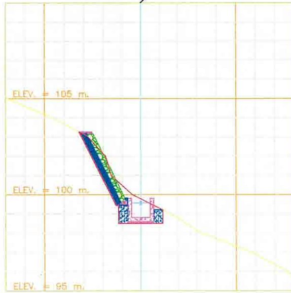
HEADRACE CHANNEL TYPICAL SECTION 5 (S = 1 : 100)
