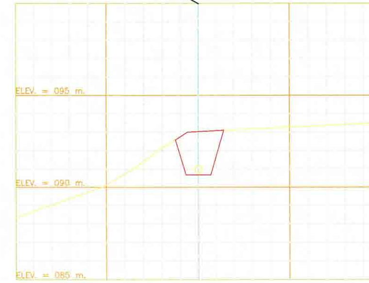
HEADRACE CHANNEL TYPICAL SECTION 3 (S = 1 : 100)
