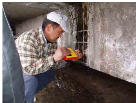
Inspection by a Schmitt hammer
