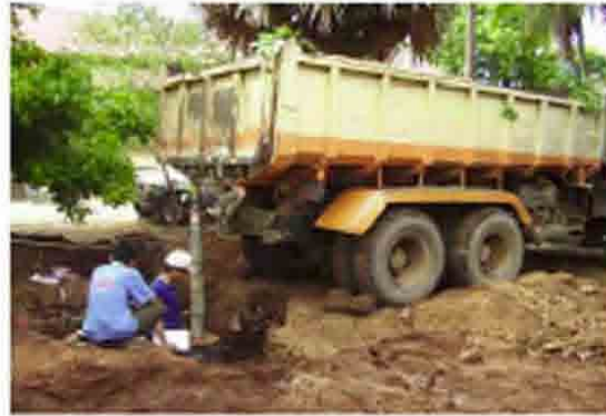
Plat load test of pit A In progress
