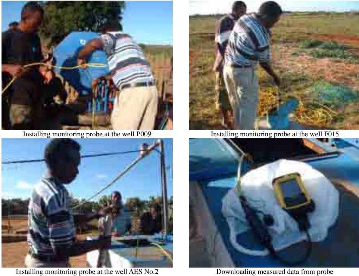
Figure 3.9.2-2 Photograph of vertical profiling
