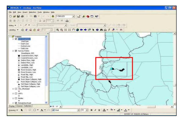
8. After the survey point is already visible, Click **Identify** tool to display the attribute for that survey point.
