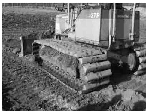
Photo 3.3 Foot Condition of Bulldozer
