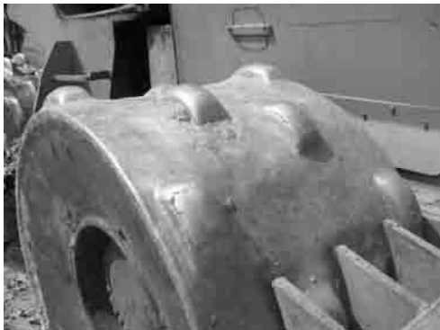
Photo 3.5 Abrasion of Driving Wheel
