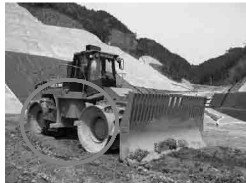
Photo 3.6 Chopper of Driving Wheel (Fukuoka)
