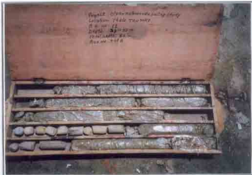
Photo 7 : Core Box BH-12; Mountain, Depth (20.00 - 35.00) m, Total Depth 40m, Clean Kathmandu Valley Study
