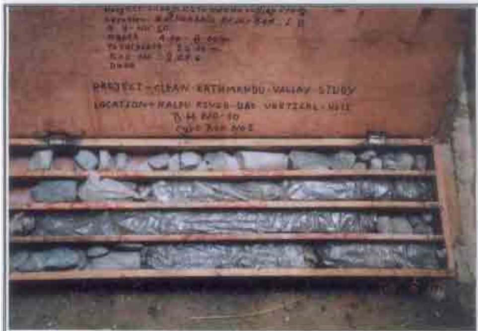
Photo 2 : Core Box BH-10, River Bed, Depth (4.00 - 8.00) m, Total Depth 25.0m, Clean Kathmandu Valley Study
