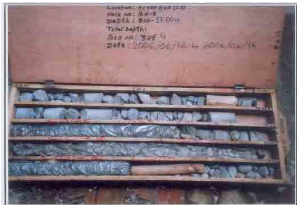
Photo 3 : Core Box BH-9, River Bed, Depth (8.00 - 13.00) m, Total Depth 15m, Clean Kathmandu Valley Study
