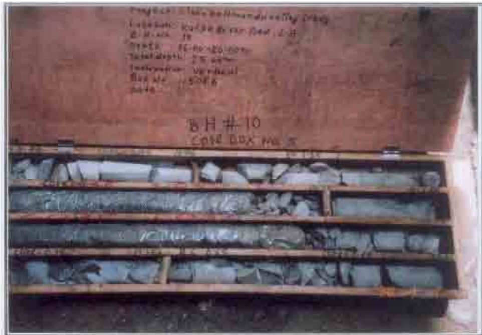
Photo 5 : Core Box BH-10, River Bed, Depth (16.00 - 20.00) m, Total Depth 25.0m, Clean Kathmandu Valley Study
