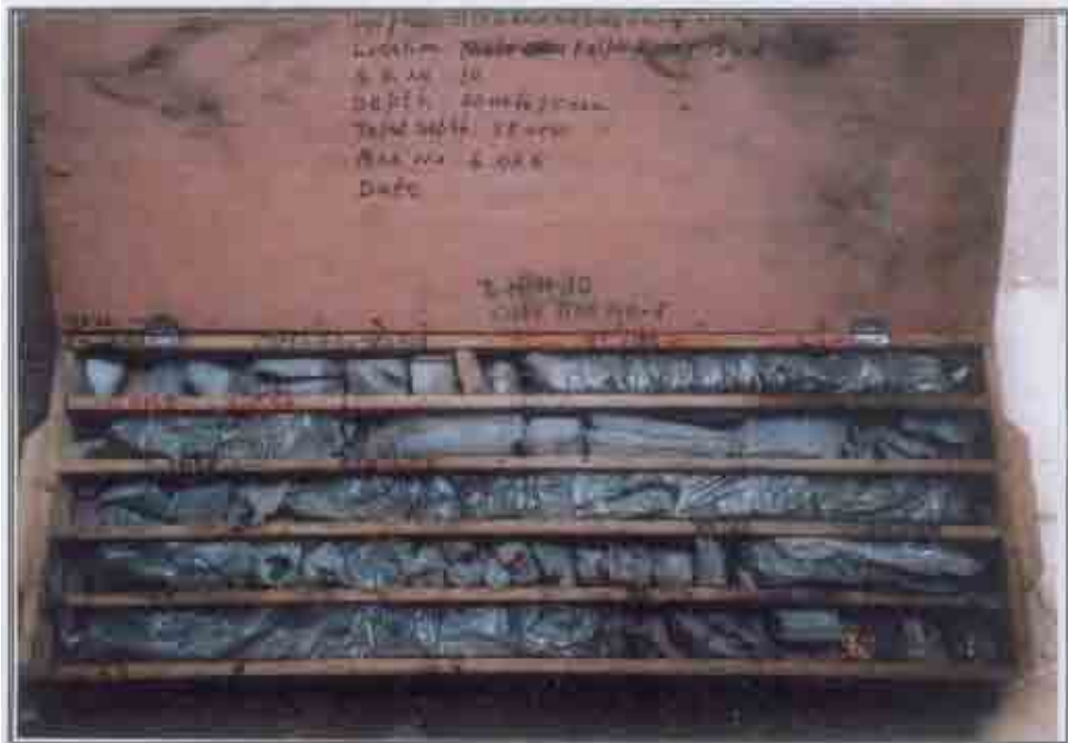
Photo 6 : Core Box BH-10, Mountain, Depth (20.00 - 25.00) m, Total Depth 25m, Clean Kathmandu Valley Study
