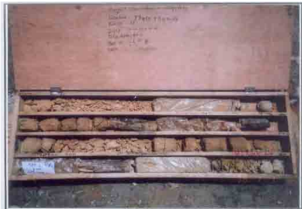
Photo 1: Core Box BH-12, Mountain, Depth (0.00 - 4.00) m, Total Depth 40m, Clean Kathmandu Valley Study
