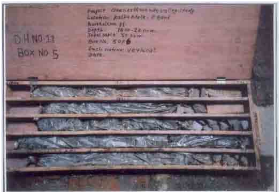
Photo 5 : Core Box BH-11, Mountain, Depth (18.00 - 23.00) m, Total Depth 30m, Clean Kathmandu Valley Study
