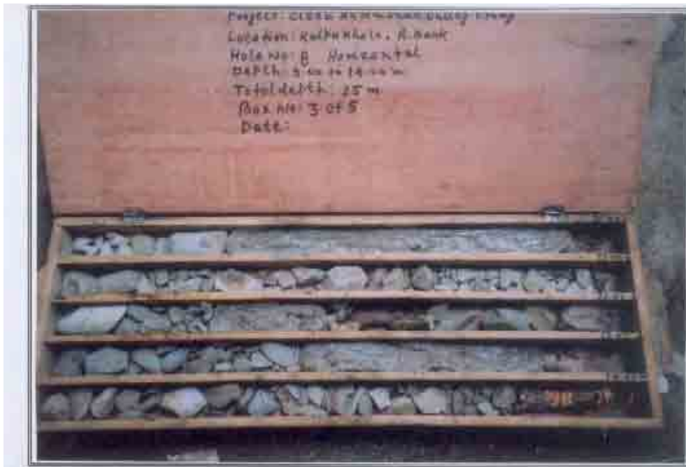
Photo.3 : Core Box BH-8, Mountain, Depth (9.00 - 14.00) m, Total Depth 25m, Clean Kathmandu Valley Study
