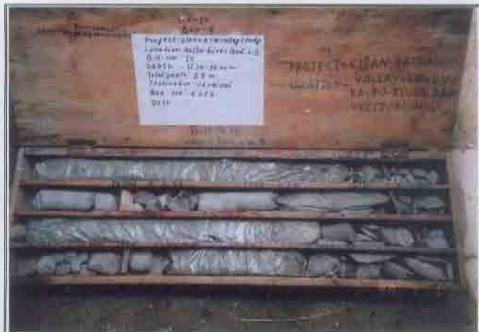
Photo 4 : Core Box BH-10, River Bed, Depth (11.70 - 16.00) m, Total Depth 25.0m, Clean Kathmandu Valley Study
