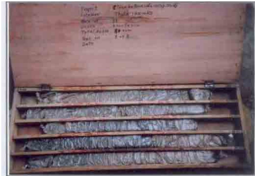
Photo 3 : Core Box BH-12, Mountain, Depth (9.00 - 14.00) m, Total Depth 40m, Clean Kathmandu Valley Study
