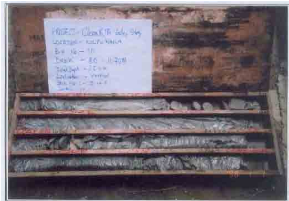
Photo 3 : Core Box BH-10, River Bed, Depth (8.00 - 11.70) m, Total Depth 25.0m, Clean Kathmandu Valley Study
