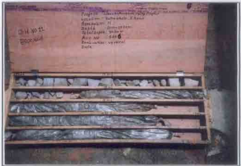
Photo 4 : Core Box BH-11, Mountain, Depth (13.00 - 18.00) m, Total Depth 30m, Clean Kathmandu Valley Study
