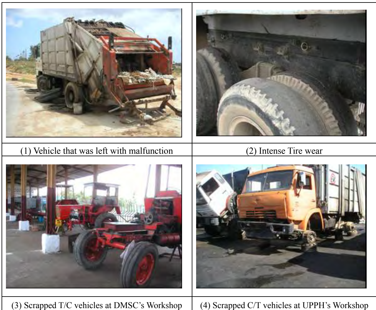
Figure 5 Typical Condition of Collection Vehicles
