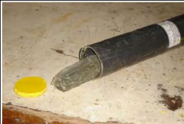
Obtained Undisturbed Sample from H1CGD Borehole
