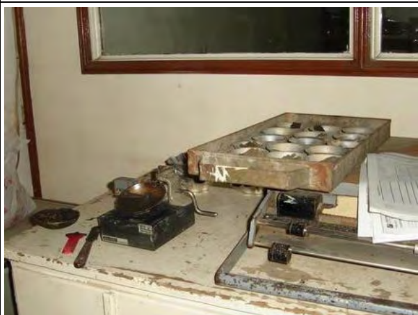
Apparatus for Plasticity Index and Testing Samples
