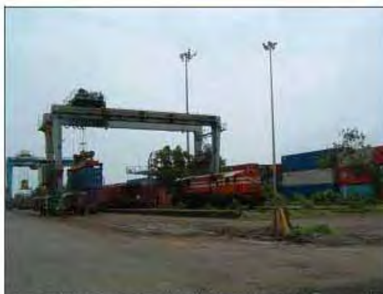
(A 20-foot container unloaded in Line No.2 is being placed by RMGC onto a trailer-truck parking alongside the railway.)
