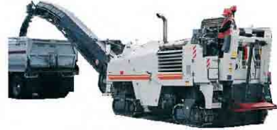
4. Asphalt Milling Machine
