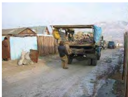
<Collection Work in the Ger Area> Dump truck is suitable for collecting heavy waste such as ashes. Loading work is very hard.
