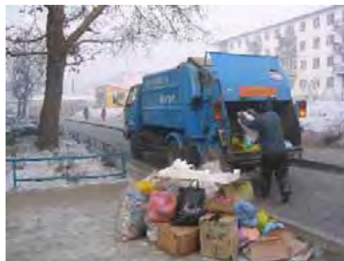
<Time & Motion Survey> The survey result revealed the collection efficiency of a Japanese secondhand collection vehicle is better than dump trucks.
