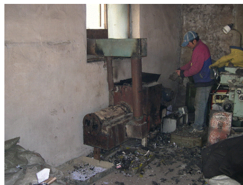
<RDF Production> RDF is produced by a locally available machine. After mixing and heating plastic and paper waste, RDF was cast by an extruder.
