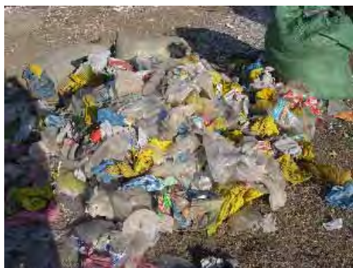
<Raw Materials of RDF> Plastic waste for RDF production. The other raw material is paper waste. Kitchen waste is not used, because it causes a problem such as fermentation, this makes RDF instable.
