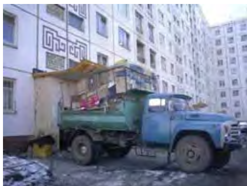
Waste generated in the Apartment area contains a lot of paper and plastic waste, so its relative density is low. A compactor truck is suitable but a dump truck is mainly used.
