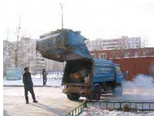
Recently secondhand compactor trucks are used, but the malfunction of the compactor reduces the collection efficiency and could cause an injury.
