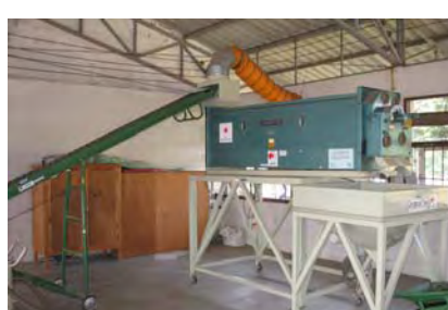
Equipment supplied from the Project at KKANRDC (Cylinder separator)
