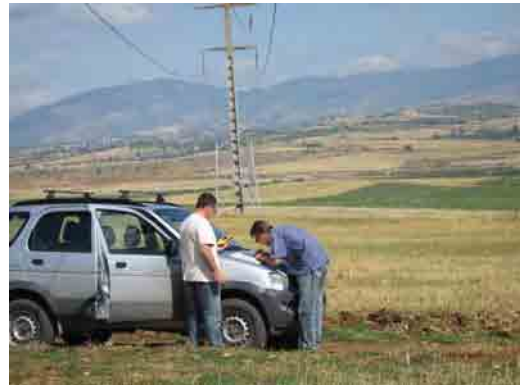
Measurement of power line coordinates by portable GPS
