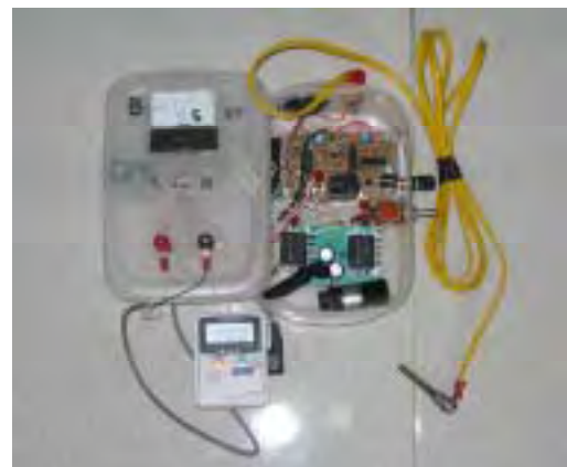
Photo 6-1-9 Coal Flow Detector
