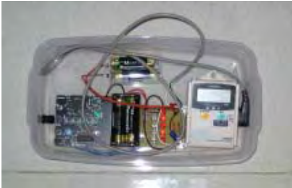
Photo 6-1-10 Motor Operation Detector
