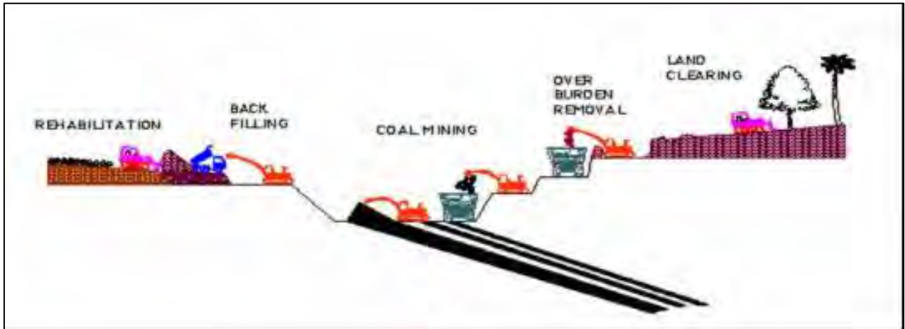
Figures 4-1-1 The sequence of the open cut mining method
