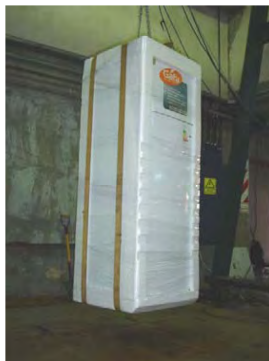
Fig 8.2.1-2 Drop Tests, Improved Product
