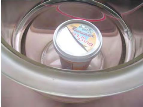
Fig. 7.3.5-11 Aluminum Foil under Normal Pressure (Curved down)
