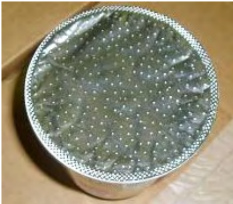
Fig. 7.3.5-14 Improved Pot Cap (with protuberances)
