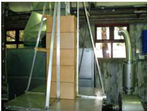
Fig. 7.3.5-3 Vibration Test on Stacked Boxes (5 Layers) - Bottom Box
