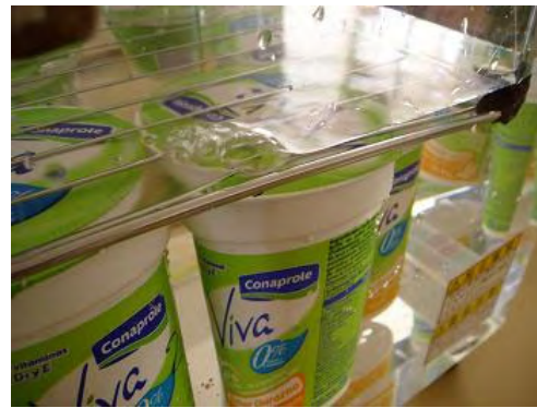
Fig. 7.3.4-6 Bubbles during Tightness Test
