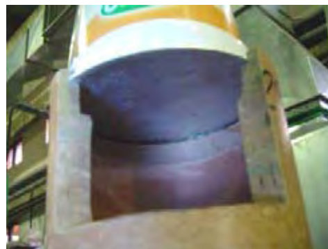
Fig. 7.3.5-10 Aluminum Lid Vibration at 20 to 40 Hz
