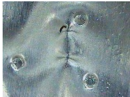
Source: JICA Study Team Fig. 7.3.5-16 Improved Cap (without protuberances) Showing Cracks
