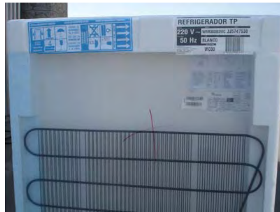
Shrinkable film meltdown. Film touching a portion of refrigerator.
