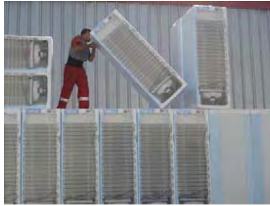
Horizontal position units loading. Cargo and personnel under dangerous procedures.
