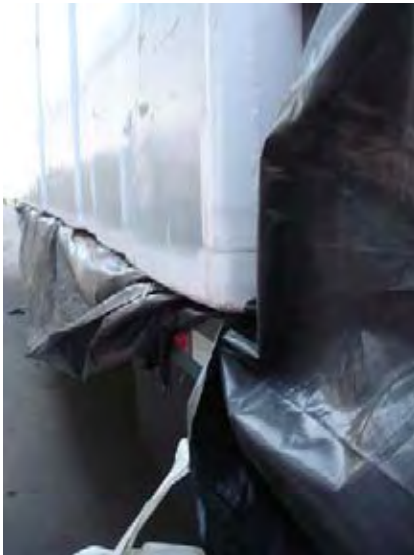
Cargo moved during transportation. EPS slightly deformed due to cargo displacement for 8cm. Source: JICA Study Team
