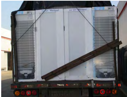
Corner support moved at the back side of truck. EPS edges are slightly damaged.
