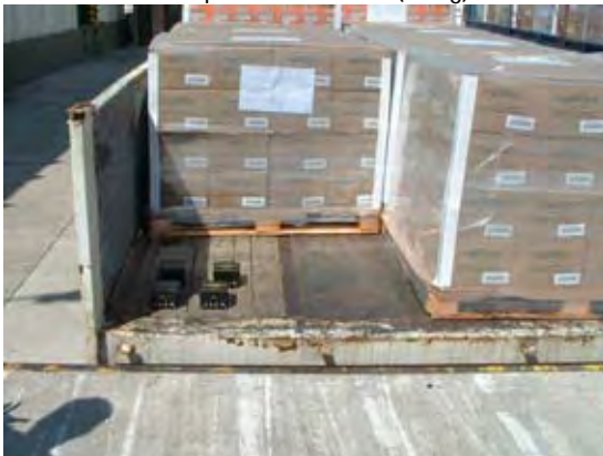
Fitting of DerSmart Sensors in the truck
