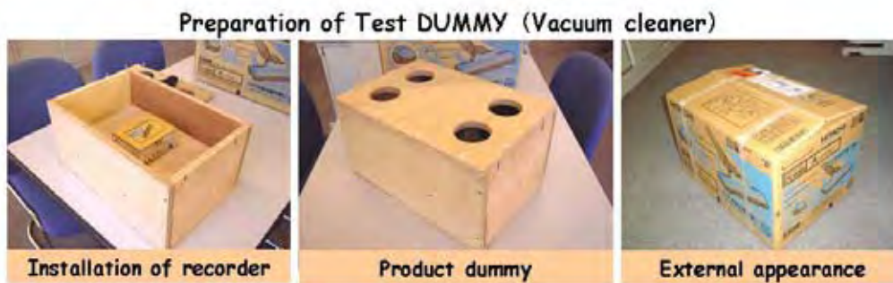
Fig. 3.2-14 Dummy Cargo for Impact Testing (vacuum cleaner)
