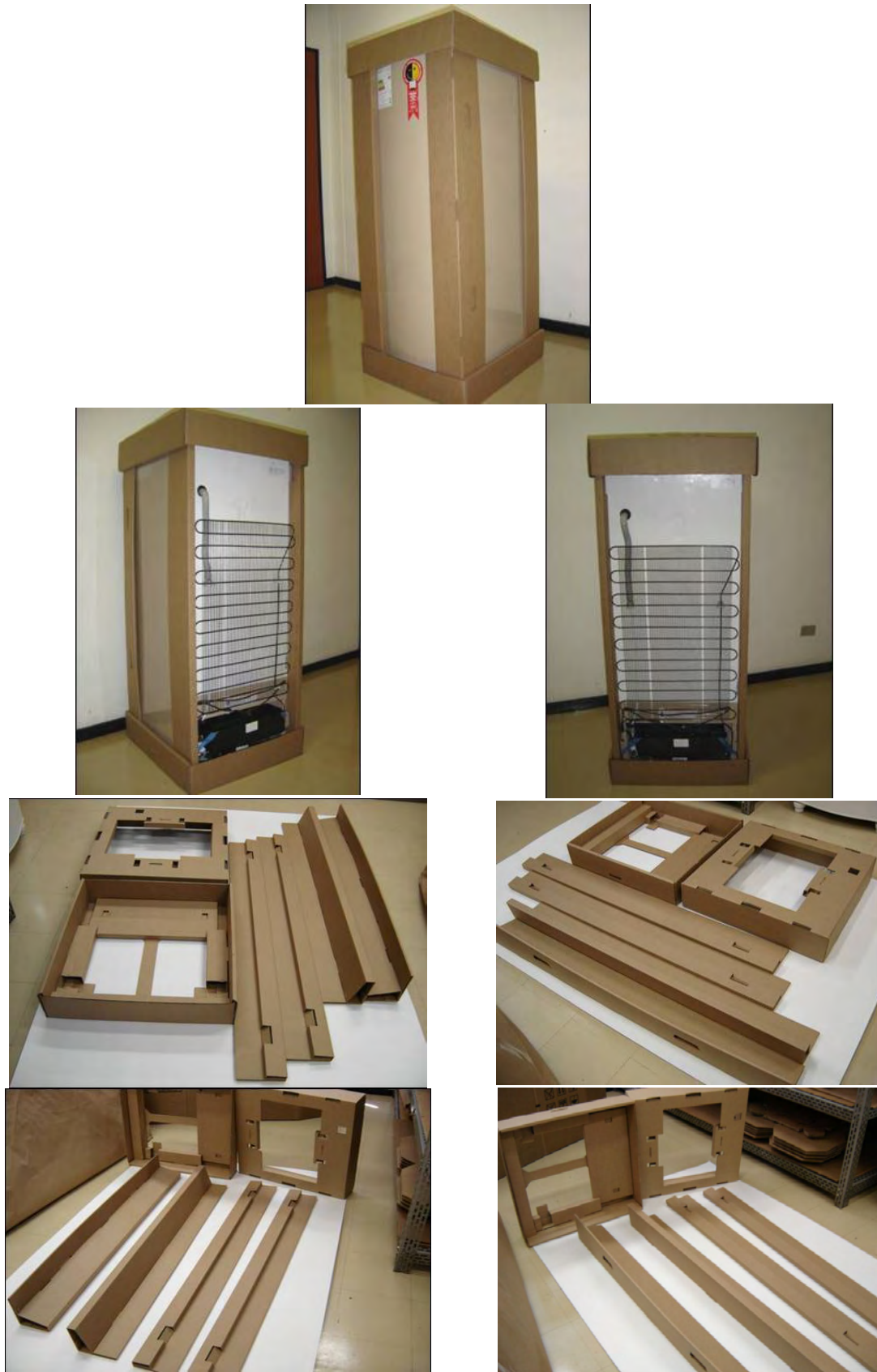
Fig. 8-4 Pilot Packaging by using Cardboard
