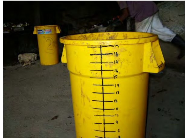
The reduced sample was placed in plastic containers calibrated to register its volume and weight.
