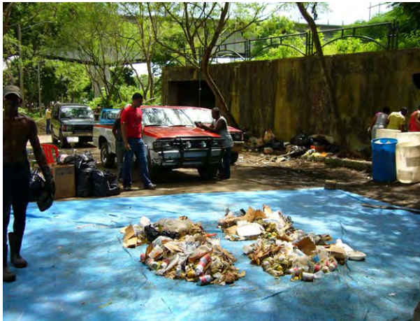
After mixing them adequately, the waste was divided in four segments of approximately the same size.
