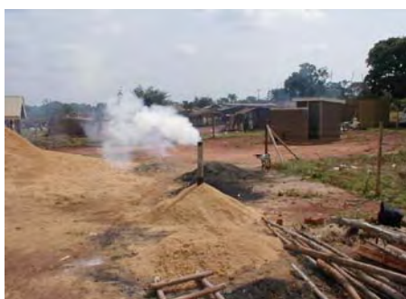
Photo5.1 Carbonized Husk Making Methods
