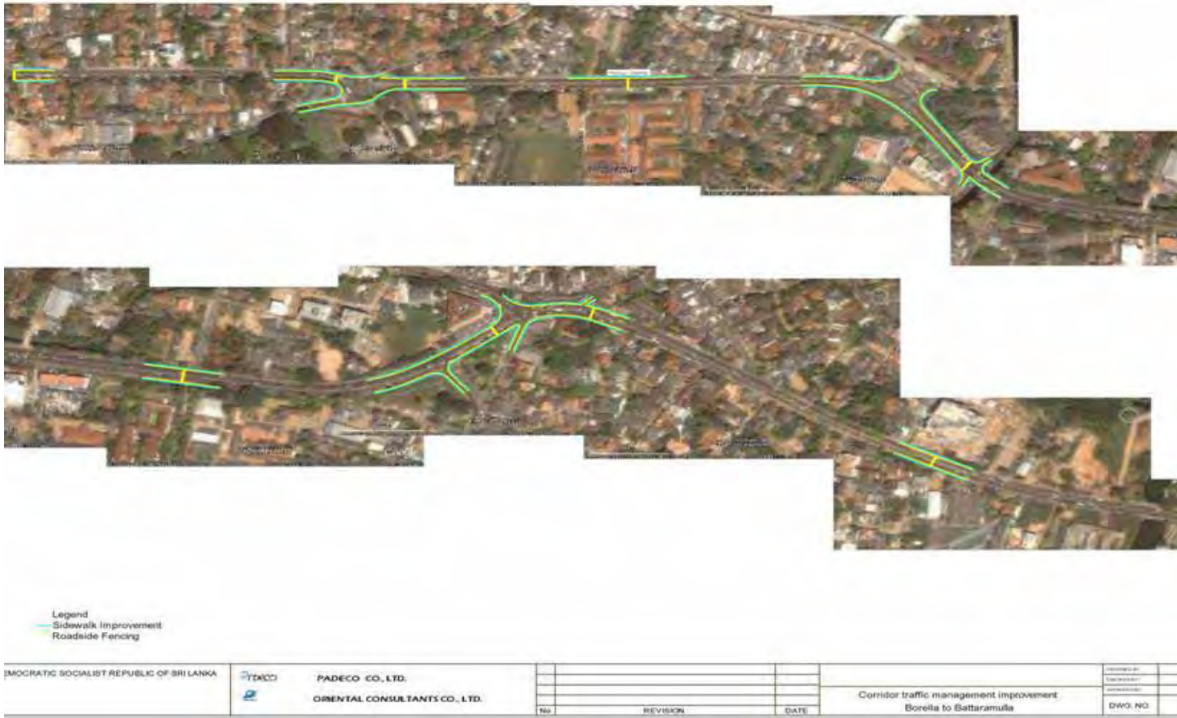
Figure A36.3 Proposed Corridor Improvements A0 from Borella to Battaramulla Part I
