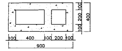
6 PROTECTION DUCT BOX SPACE TYPE - F SCALE 1:30
