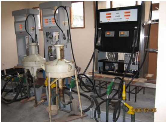
Photo 5.7.2.5 Fuel oil calibration stand
