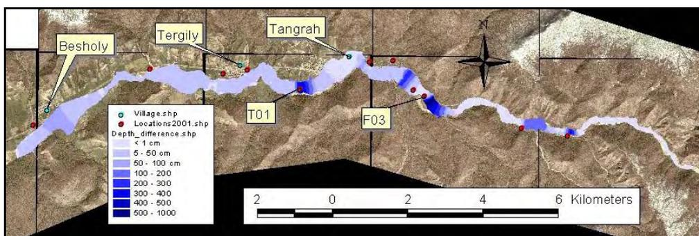
Figure 8.14 Comparison map (maximum depth with debris minus maximum depth without debris) for the 100 year flood.
