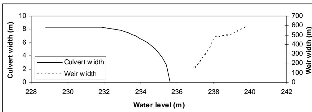
Figure 7.2 Level-width curves for 14 Metry Bridge (culvert and weir).
