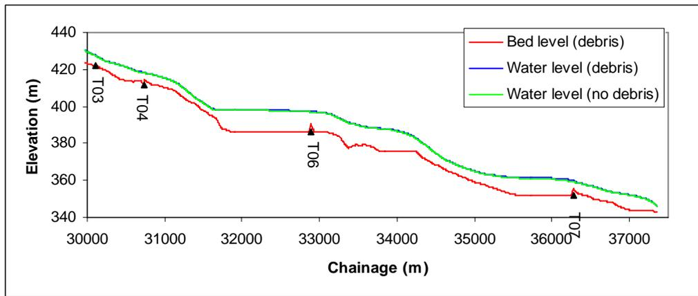
**Figure 8.9** Profiles of the maximum water level (with and without debris) and maximum bed level (with debris) for the debris flow simulation with the 100 year event, downstream part of the local debris model.
