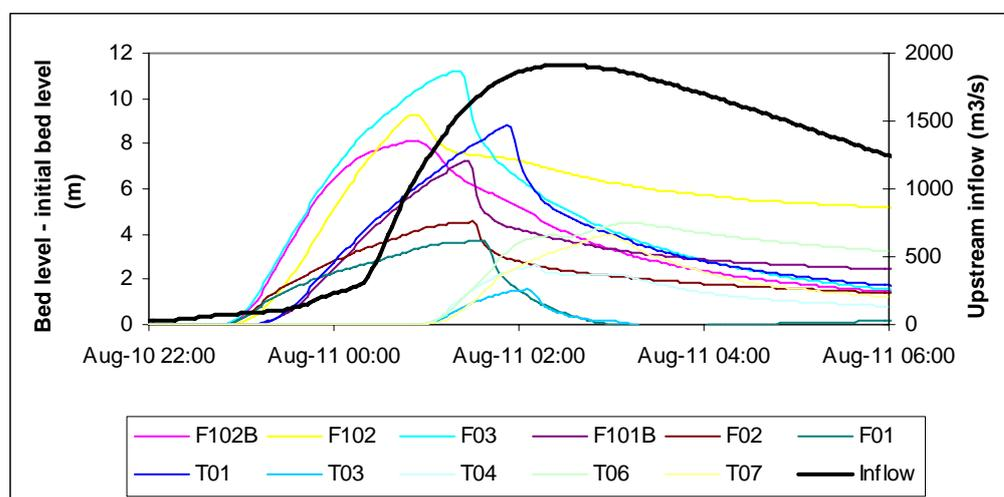
**Figure 8.7 Temporal development of the bed level minus the initial bed level for all the debris dams shown along with the water inflow.**
