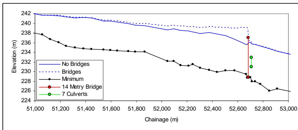
**Figure 7.3 Backwater calculation at 14 Metry (and 7 Culverts) Bridge. The inverts (culvert and road) are shown for each bridge. It is seen that 14 Metry backs the water up more than 1 km.**
