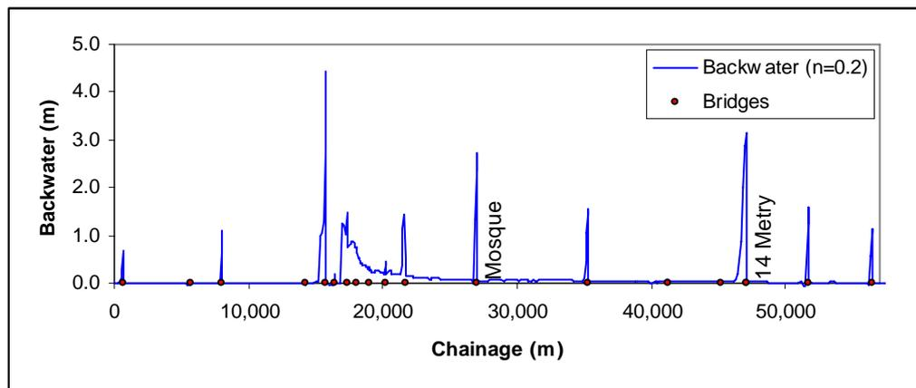
**Figure 7.12** Bridge backwater (water level with bridges minus water level without bridges) calculated with “Mosaic” MIKE 11 model with a Manning  $n=0.20 \text{ s/m}^{1/3}$ , and modified level-width curves that match the cross-sections.
