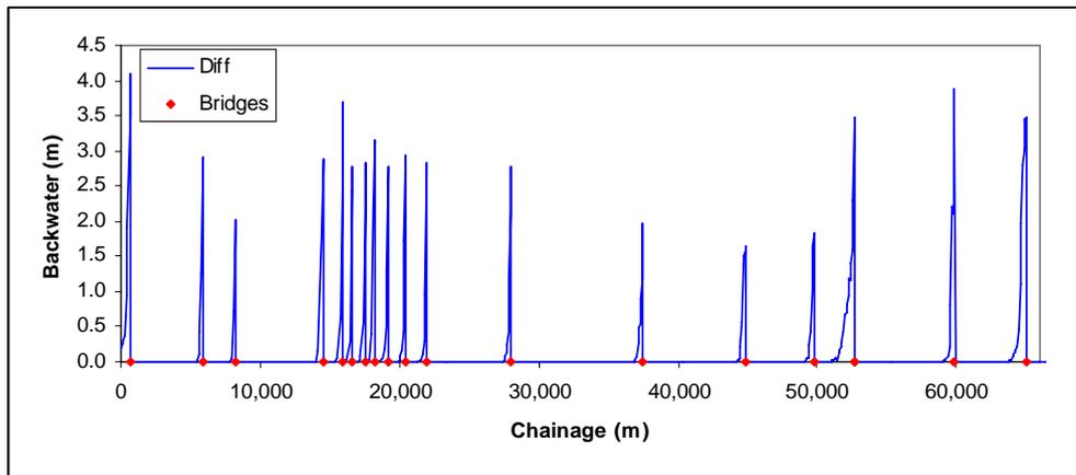
Figure 7.5 Backwater curves for all 19 bridges calculated for a constant discharge of 1600 m<sup>3</sup>/s.
