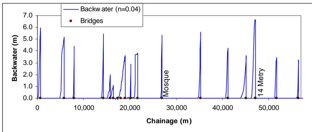
**Figure 7.9** Bridge backwater (water level with bridges minus water level without bridges) calculated with “Mosaic” MIKE 11 model with a Manning n=0.04 s/m<sup>1/3</sup>.
