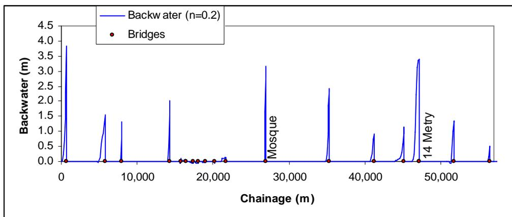
**Figure 7.10** Bridge backwater (water level with bridges minus water level without bridges) calculated with “Mosaic” MIKE 11 model with a Manning n=0.04 s/m<sup>1/3</sup>.
