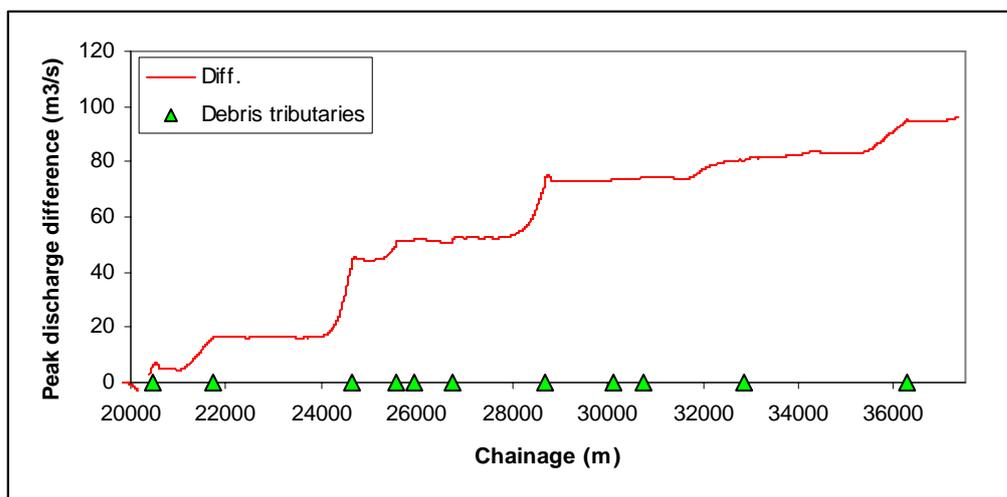
**Figure 8.12 The longitudinal variation in the difference in peak discharge (with debris minus without debris) down through the local model.**
