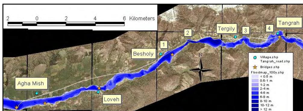
**Figure 8.5 Overtopping of Tangrah Road between 14 Metry Bridge and Tangrah determined from the 100 year flood map and the location of Tangrah road (from 1:25,000 map confirmed with GPS points). Four locations (1-4) are identified from this map.**
