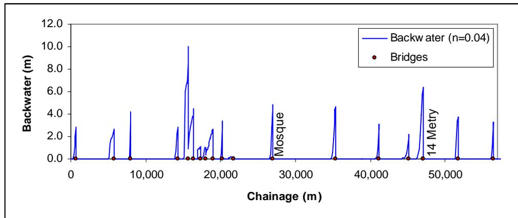
**Figure 7.11** Bridge backwater (water level with bridges minus water level without bridges) calculated with “Mosaic” MIKE 11 model with a Manning  $n=0.04 \text{ s/m}^{1/3}$ , and modified level-width curves that match the cross-sections.
