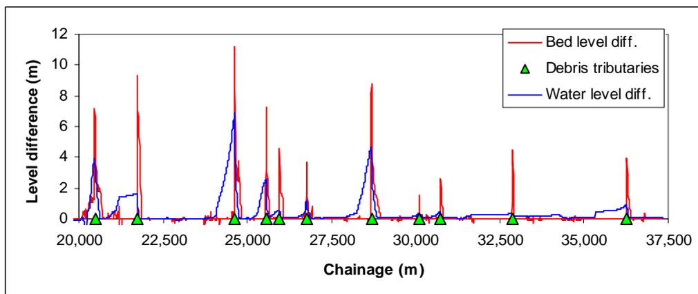
**Figure 8.10** Difference in maximum bed and water level caused by the presence of debris flow (100 year event).
