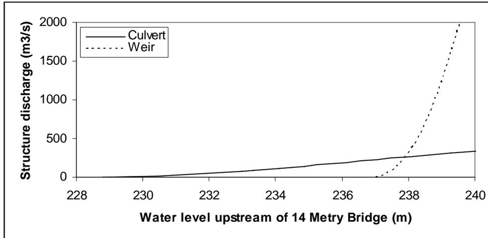
Figure 7.4 Q-H relations for the two structures (culvert and weir) comprising 14 Mety Bridge.
