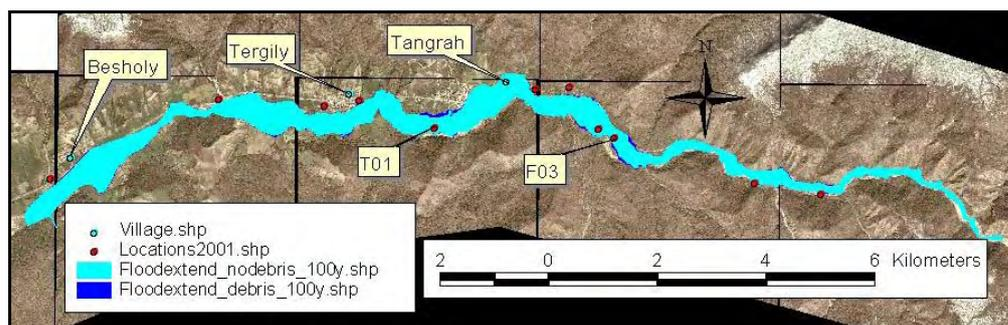
**Figure 8.15 Flood extend with and without debris flow for the 100 year flood.**
