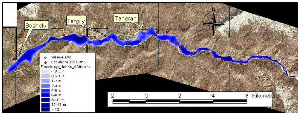
Figure 8.13 Flood map for the local model (100 year flood, maximum flood level) with debris flow included.
