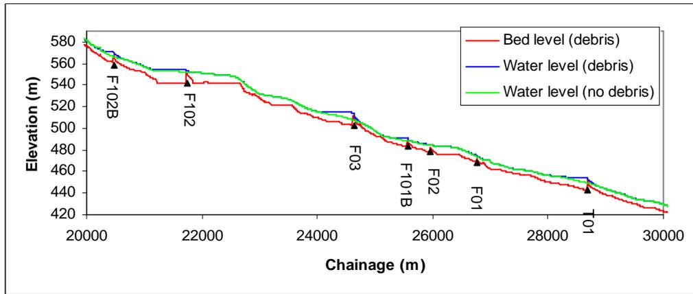
**Figure 8.8** Profiles of the maximum water level (with and without debris) and maximum bed level (with debris) for the debris flow simulation with the 100 year event, upstream part of the local debris model.
