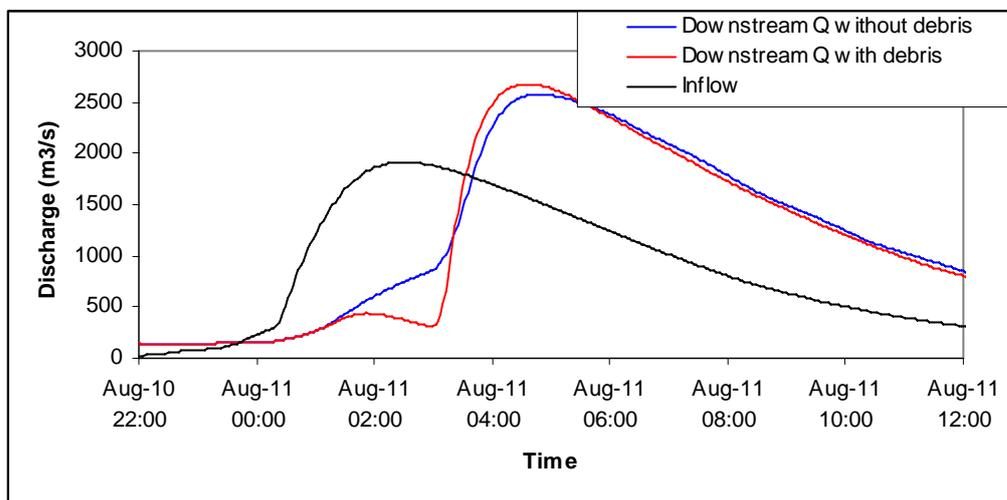
**Figure 8.11 Temporal variation of the downstream discharge in the local debris model with and without debris flow included.**
