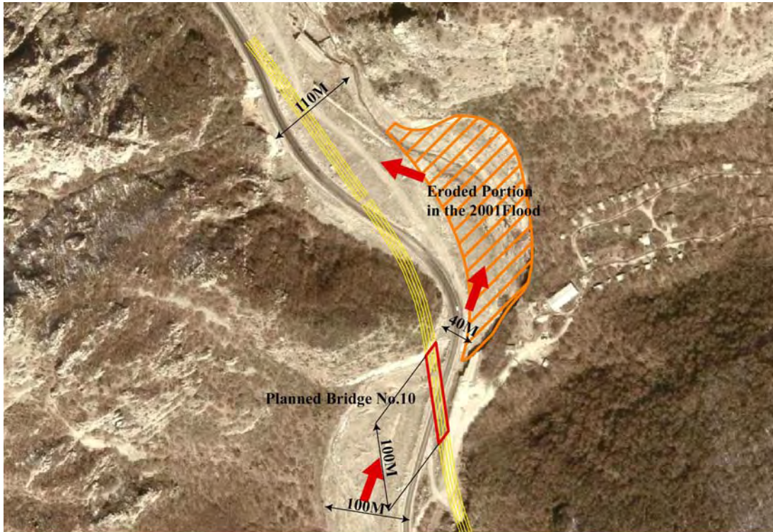
Figure A6-11 Satellite Image with Road Plan (Location of Planned Bridge No.10)
