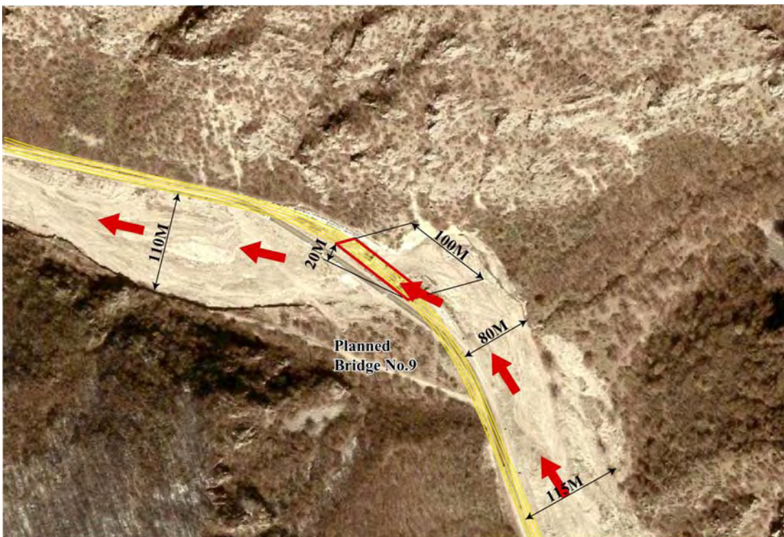
Figure A6-10 Satellite Image with Road Plan (Location of Planned Bridge No.9)
