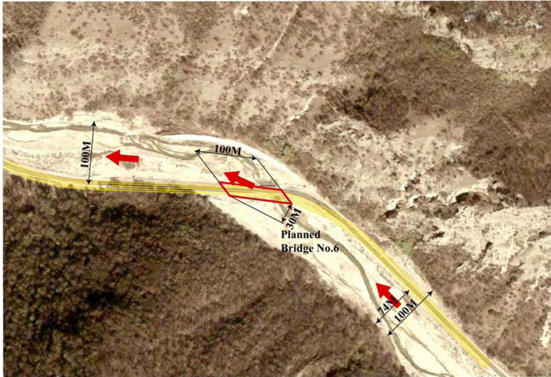
Figure A6-7 Satellite Image with Road Plan (Location of Planned Bridge No.6)
