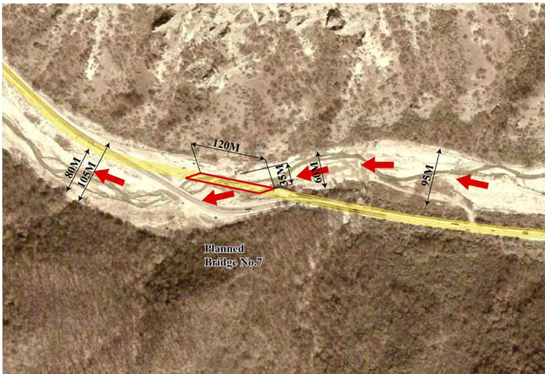
Figure A6-8 Satellite Image with Road Plan (Location of Planned Bridge No.7)
