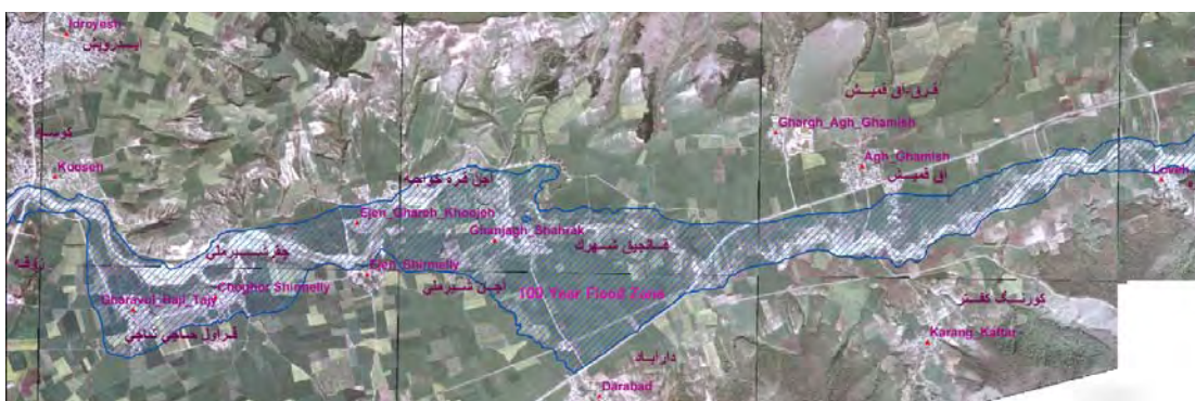
Fig. II.26 Example of Hazard Map in 100-Year Flood between Kalaleh Bridge and Lovah Village
