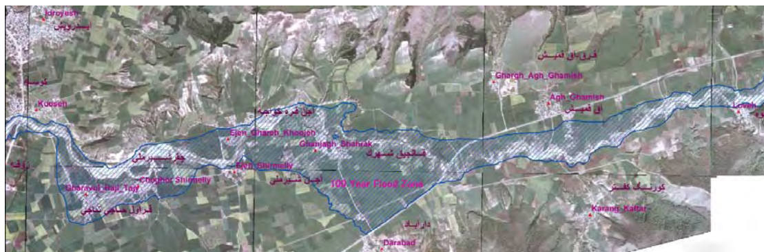
Fig. 6.5 Hazard Map in 100-Year Flood between Kalaleh Bridge and Lovah Village
