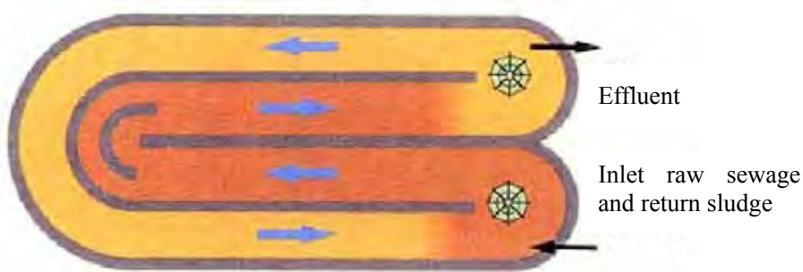
Figure M62.3.2 Illustration of Oxidation Ditch Process
